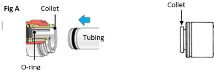
The cartridge body has high pressure Quick Connect fittings (Collets), pre-moulded into each end. Check the flow direction arrows on the new cartridge and reattach the tubing simply by pushing the nylon pipe from the clamp into fitting "A" and then the pipe from the faucet into fitting "B". The pipe should go approx. 20 mm into the fitting then stop. Check that the tube is securely held by the collets.
